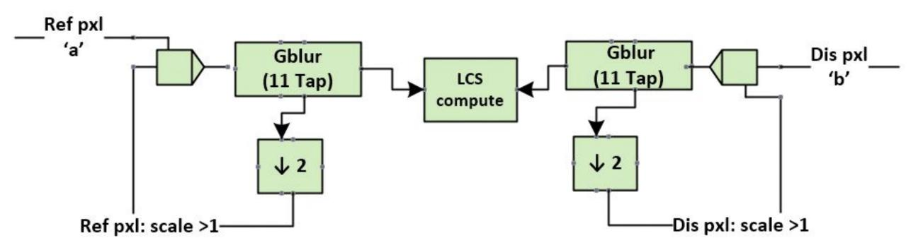
These components are smoothened using a 11 tap Gaussian blur filter before computing L and CS
